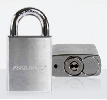
A strong and durable padlock, suitable for a wide range of commercial or industrial applications. Specifically developed to accept an ABLOY cylinder, the PL6B Padlock offers the flexibility to be set up with latching function, where the key can be removed with the shackle in the open position, or deadlocking function, where the key is retained and can only be removed with the shackle in the locked position.
